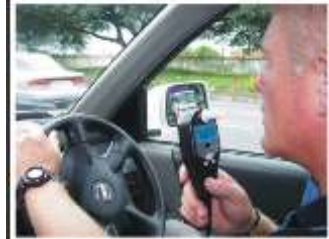
Driver providing breath sample to release Vehicle Blocking System
